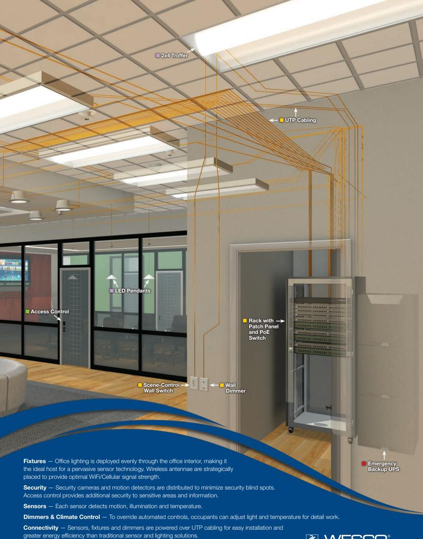
**PoE Switch** — Converts AC power to low-voltage DC power.
